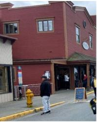
Photo 3 - A fire hydrant, building columns and shop signs reduce effective sidewalk width on Lincoln Street
